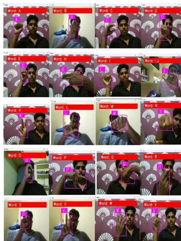
Figure 3. Detection of sign language alphabet gestures using the proposed HandSpeak framework.
